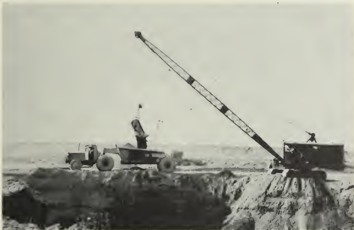
A, PACIFIC COAST AGGREGATES, INC., CENTERVILLE, ALAMEDA COUNTY Mining gravel with dragline for concrete-aggregate. Fenelon F. Davis, photography, 1949.
